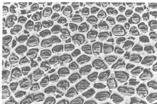
Figure 2 Scanning electron micrograph of the central region of the tooth of *Psammechinus miliaris*. The tooth was embedded in resin, ground down to a plane normal to the long axis of the fibres, polished and etched briefly in dilute hydrochloric acid. The mean diameter of the fibres is about 6  $\mu\text{m}$ . Note the parallel lines on the etched surfaces of the fibres. These show that the fibres have all essentially the same crystallographic orientation.
