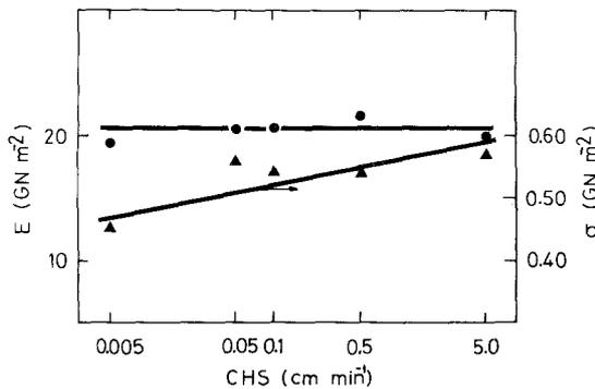
Figure 1 Values of the longitudinal modulus and ultimate strength as functions of the cross-head speed (CHS). The results at 0.05 cm min<sup>-1</sup> are taken from [6], and  $V_f = 0.39\%$ .
