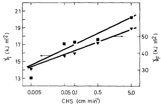
Figure 2 Values of the longitudinal fracture surface energy and work of fracture as functions of the cross-head speed (CHS). The results at 0.05 cm min<sup>-1</sup> are taken from [6], and  $V_f = 0.39\%$ .
