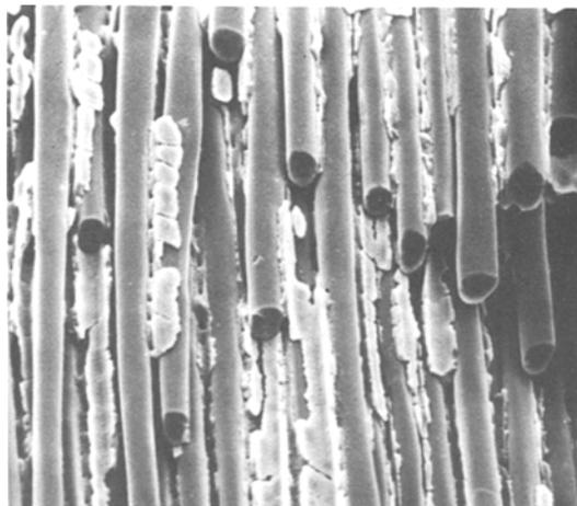
Figure 1 Scanning electron micrograph of the central region of the tooth of *Psammechinus miliaris*. The tooth was fractured and then vibrated in an ultrasonic bath for 2 min. The fibres are about 6  $\mu\text{m}$  in diameter.
